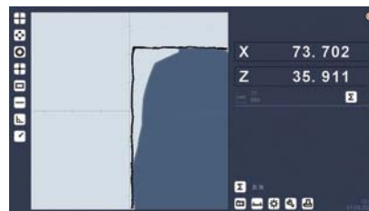
scanning the maximum profile of cutting tools
