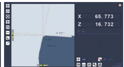
dynamic crosshair automatically adjusting as X and Z axis move, and the cutting tools can be quickly measured through the dynamic crosshair.
